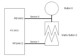
In the system there are 2 sensors, 1 button and 1 matrix button. Thus in mTouchConfig.h MTOUCH\_SENSORS\_NUMBER must be set to 2, MTOUCH\_BUTTONS\_NUMBER and MTOUCH\_MATRIXBUTTONS\_NUMBER must be set to 1. All IOs connected to sensors must be set as ANALOG in the application (see PCFGx, ANSx or ANSELx registers description in PIC Microcontroller datasheet ).
