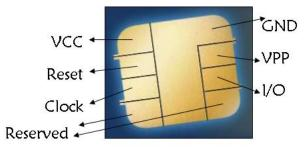
I/O: Input or Output for serial data to the integrated circuit inside the card.
