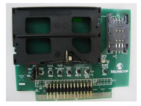
5. Insert the J2 slot of SC (Smart/Sim Card) PICTail card into J5 port of Explorer 16 board. Make sure that the Smart Card Connector is facing towards the Explorer 16 board. Insert the Smart Card in SC PICTail board.
